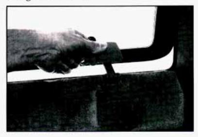
To open your swing-out windows, pull up on the latch and push the window out.
